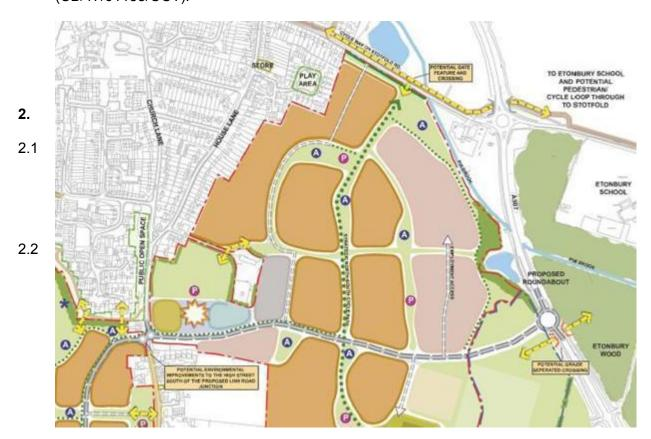
2.3 The signalised crossings have been designed as Toucan type crossings. They have been located along key desire lines that will come forward once the masterplan is developed, namely routes to the local centre, along the strategic north - south cycle route and the central bus stop. This is considered an acceptable reason for choosing these locations. Cycle and pedestrian routes to connect to these crossings will be considered in detail by officers as part of planning application CB/01277/OUT.
